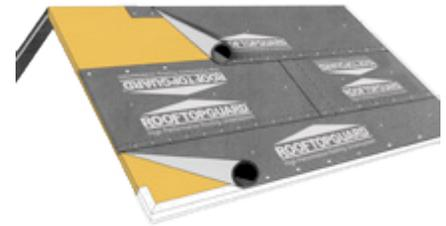
**FASTENING METHOD:** RoofTopGuard II must be attached to the structural Roof Deck Material using Plastic or Steel Cap roofing nails, having a minimum of 1" diameter cap, spaced at 12" on vertical and 14" on horizontal. All Plastic, or Steel Caps, must be attached flush with the underlayment surface and nails must be fastened at a 90 degree angle to the deck. Follow the nailing pattern, which is marked by X's on the product.
